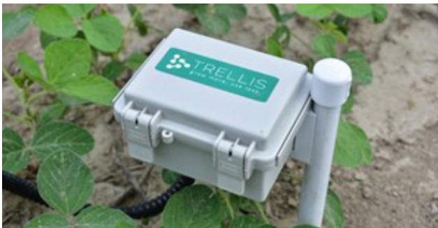
Figure 3.34 and Figure 3.35. Telemetry units
