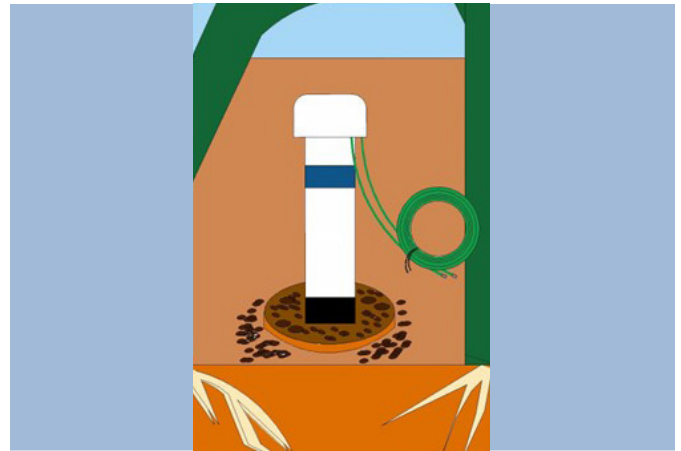
Figure 3.30. Place the sensor in the hole, packing down and mounding soil.
