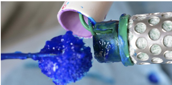
Figure 3.16. Apply ABS-PVC cement to the sensor collar.
